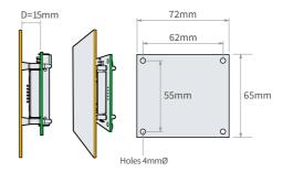
The recommended material situated in front of the 331 is 4mm thick polycarbonate.
