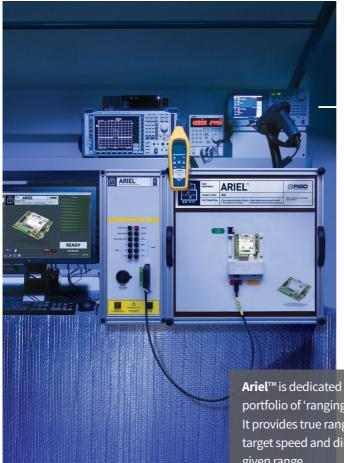
Ariel<sup>™</sup> is a bespoke set of test equipment designed and developed by AGD Systems. It is dedicated to the testing of the AGD portfolio of 'ranging' FMCW vehicle radars. 100% of the 331units manufactured at AGD are Certified by Ariel.
