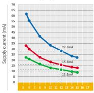
Supply voltage (v) FIG 1: SUPPLY CURRENT **VS**. SUPPLY VOLTAGE
