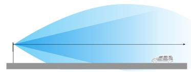
The radars front face should be 90<sup>0</sup> to the road surface, inclines in the road surface should be catered for by adjusting the 331 radars mounting angle.
