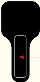
Battery compartment cover - takes 2x AA batteries
