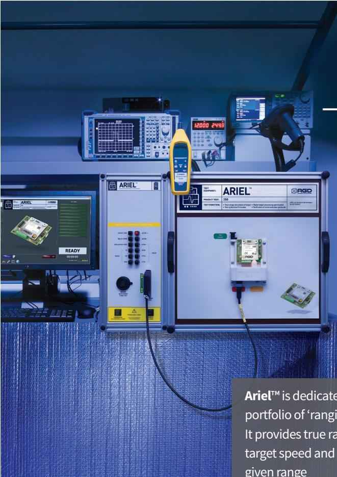
Ariel™ is a bespoke set of test equipment designed and developed by AGD Systems. It is dedicated to the testing of the AGD portfolio of 'ranging' FMCW vehicle radars. 100% of the 331 units manufactured at AGD are Certified by Ariel.
