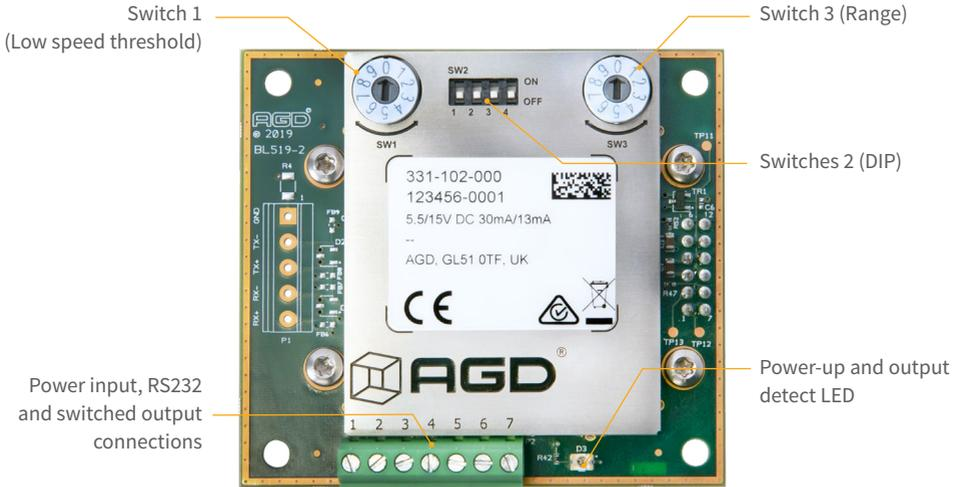
\* SW1 and SW3 can only be used to set the low speed threshold and range on switched output 1
