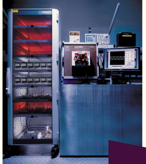
Saturn<sup>™</sup> is a bespoke set of test equipment designed and developed by AGD Systems. It is dedicated to the testing of the 307 detector range and 100% of these units manufactured at AGD are Certified by Saturn.
